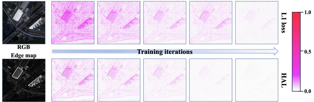
Figure 4. Comparison of gradient contribution: L1 Loss versus HAL across training iterations. The darker the color in the gradient map, the greater the proportion of its gradient contribution. The training sample is from the GF2 dataset, where the spectral response range for gradient calculation is 520-590nm.
