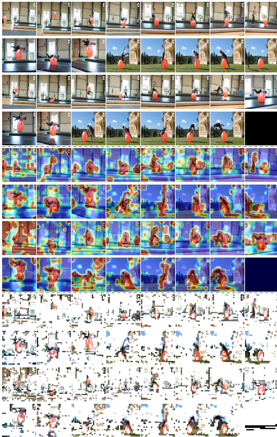
Figure 8. Visualization of token merging. Top: Frames of the input video. Middle: Residual energy maps derived from metadata. Bottom: Video frames after token merging, where merged tokens are visualized as blank blocks.
