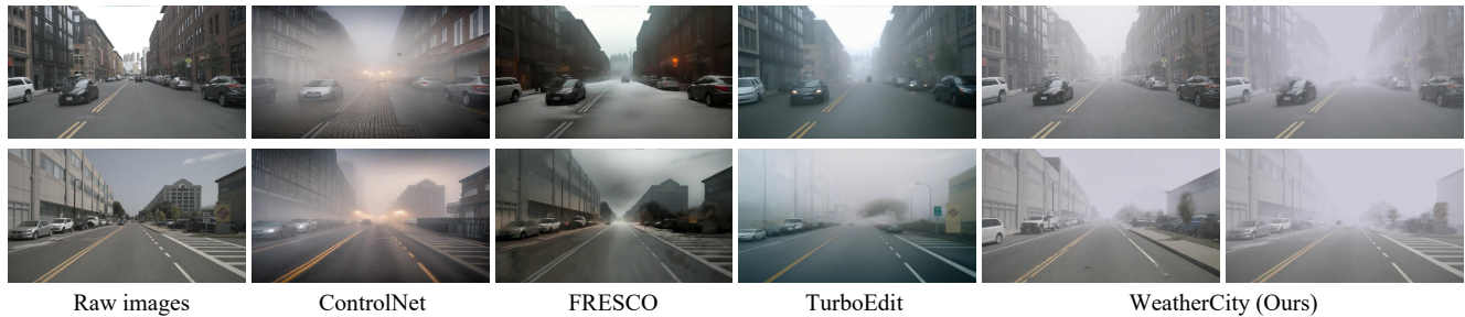
Figure 6. Qualitative comparison of foggy weather on the nuScenes Dataset. WeatherCity achieves a natural atmospheric haze that smoothly obscures distant objects, exhibiting fewer artifacts than TurboEdit or other baselines.
