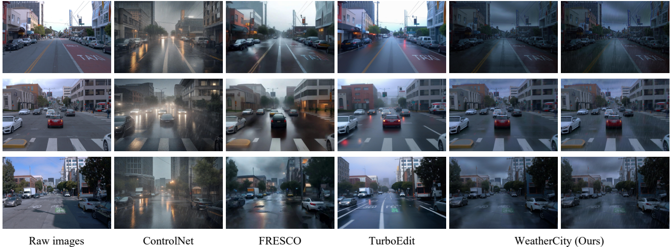
Figure 1. Qualitative comparison of rainy weather on the Waymo Open Dataset. Our model excels at capturing complex lighting interactions and environmental changes induced by rain, providing a higher level of physical realism.
