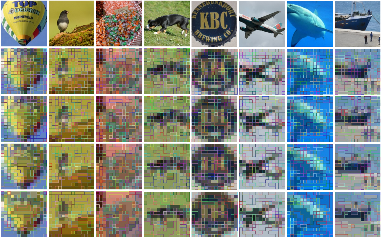
Figure 6. Visualization results of our SAD-TM on DeiT-Tiny model under the FLOPs of 0.8G. The images in each row represent the original image and the corresponding intermediate merging results after the third block, the sixth block, the ninth block, and the final merging results, respectively.
