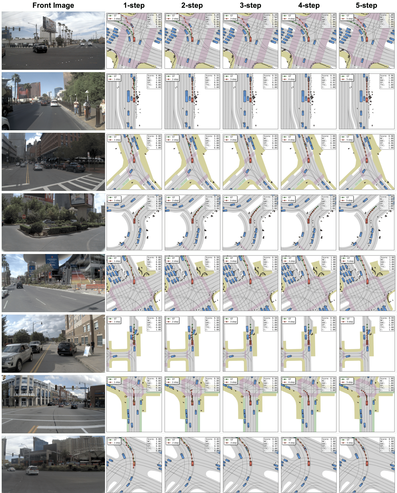
Figure 4. For relatively complex scenarios on NAVSIM, our model generates reasonable results through a 5-step coarse-to-fine trajectory prediction process.
