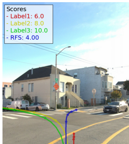
(c) Floored scores (RFS=4) are assigned because predictions are far from any of the rater-specified trajectories.
