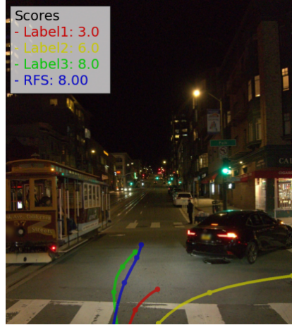
(a) The model predicted future trajectory (blue) aligns well with one of the rater specified trajectories. The corresponding flat scores are assigned as the predictions fall within the trust region.
