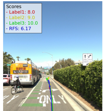
(b) The model predicted future trajectory (blue) deviates from rater specified trajectories. Since the predictions fall outside the trust regions, final scores are exponentially decayed.
