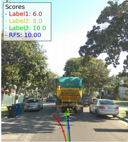
(a) The model predicted future trajectory (blue) aligns well with one of the rater specified trajectories. The corresponding flat scores are assigned as the predictions fall within the trust region.
