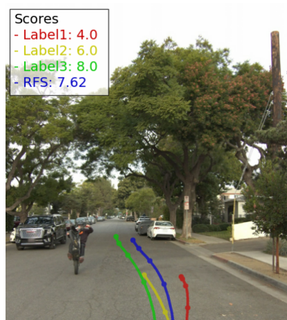
(b) The model predicted future trajectory (blue) deviates from rater specified trajectories. Since the predictions fall outside the trust regions, final scores are exponentially decayed.
