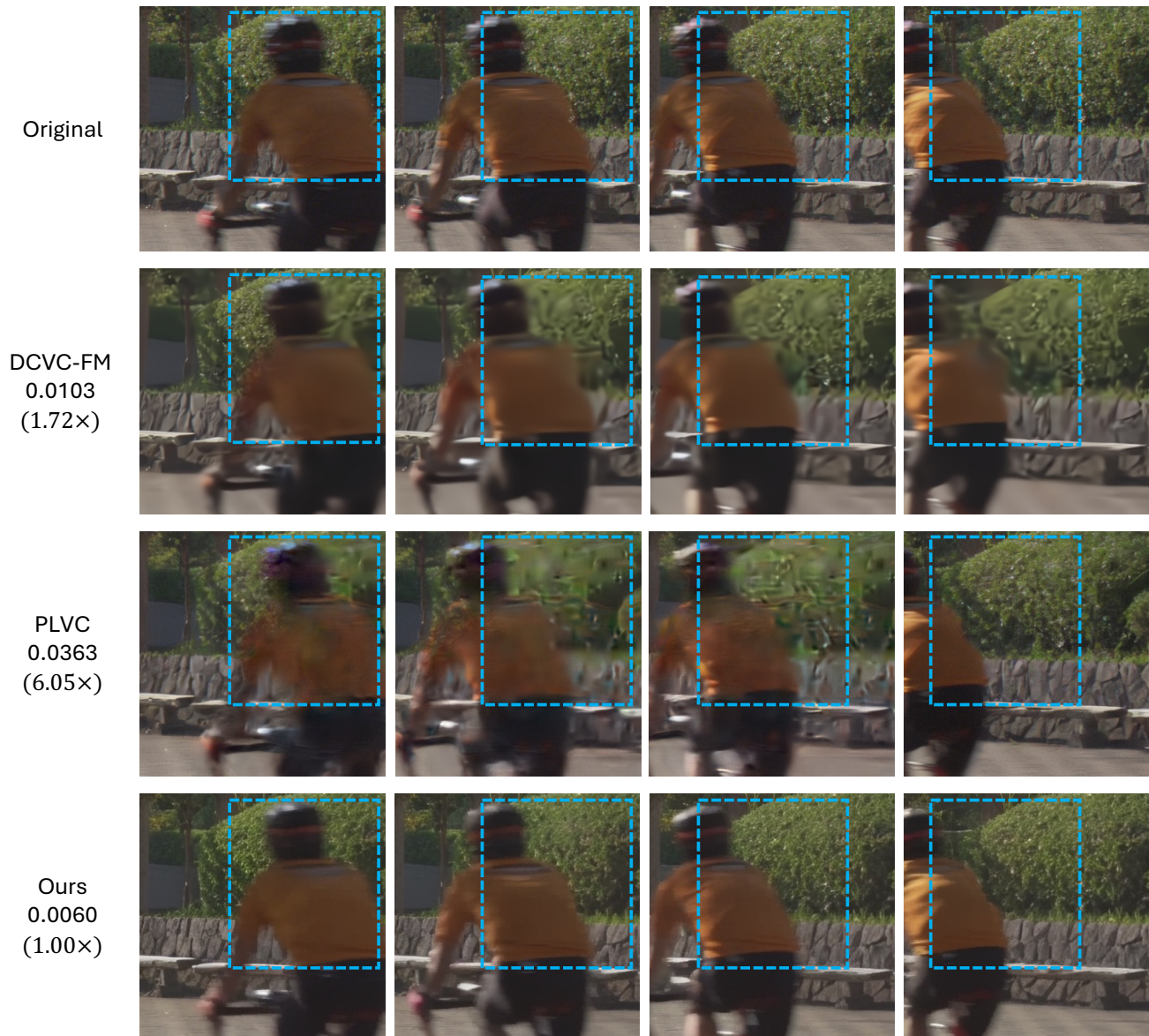
Figure 13. Additional visual examples in a motion scenario across neural codecs. The proposed S^2VC synthesizes consistent texture on the background trees, unaffected by the moving subject. In contrast, DCVC-FM generates blurry details, while PLVC produces jitter artifacts on both the subject and background, resulting in temporal inconsistencies.
