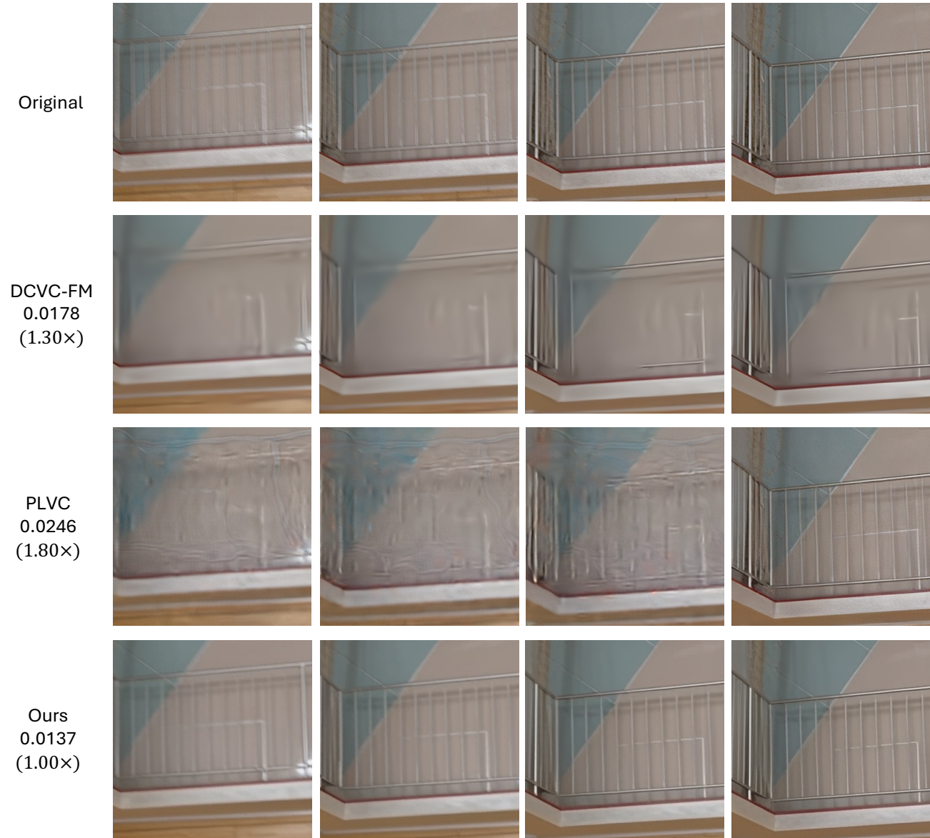
Figure 11. The proposed S^2VC accurately reconstructs the railing structure, whereas the neural codec DCVC-FM fails to recover its geometry, and the perceptual codec PLVC introduces additional temporally inconsistent noise.
