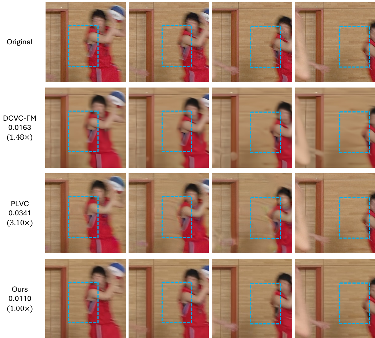
Figure 12. Additional visual examples in a motion scenario across neural codecs. The proposed S^2VC delivers the clearest and most temporally consistent texture on the wall, even as the subject moves over it. In contrast, DCVC-FM generates blurry details, while PLVC produces distorted textures that are inconsistent over time.
