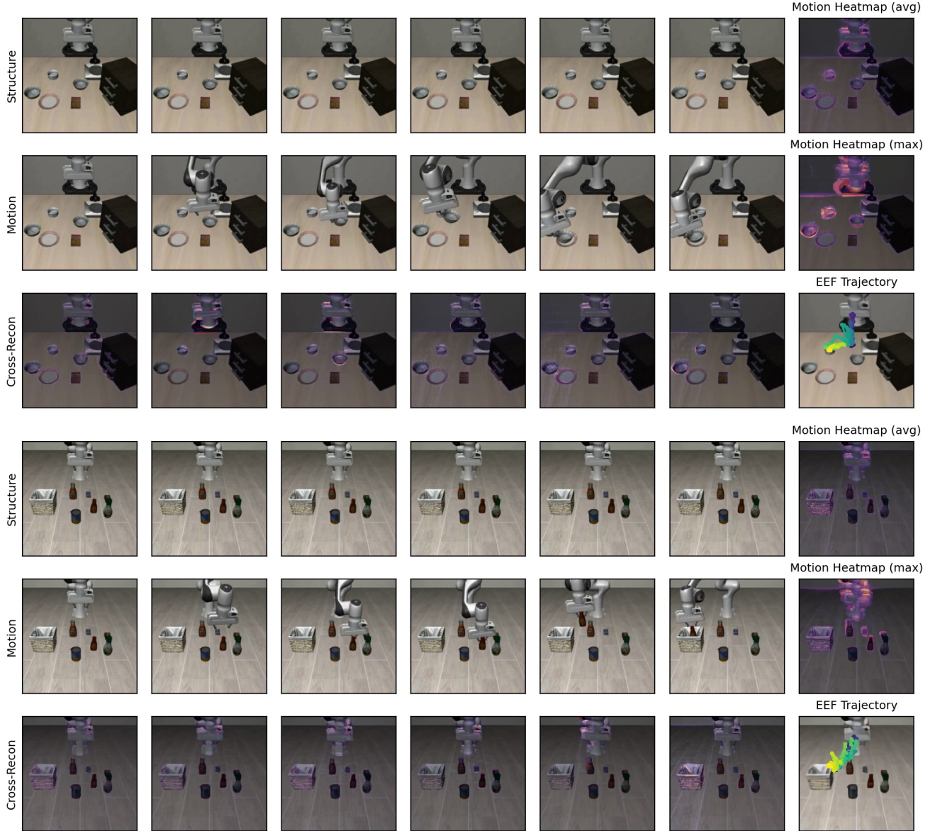
Figure 2. Cross-Recon visualization on LIBERO [12]. The first six columns show temporally sampled frames from three rows: Structure (top), Motion (middle), and Cross-Recon (bottom). The Cross-Recon videos are generated by combining the static appearance from the Structure video with the motion representation extracted from the Motion video, revealing the transferred motion patterns. Each Cross-Recon frame is overlaid with a motion heatmap to highlight dynamic regions. The last column presents three summary maps: motion heatmaps obtained by averaging and maximizing per-frame absolute differences between Cross-Recon and Structure, and the end-effector trajectory estimated from the motion regions.
