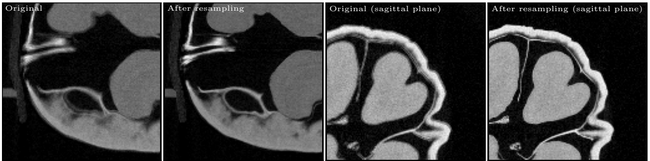
Figure 9. Comparison of FDK reconstructions using all 720 projections of FIPS [29] before and after center of rotation correction. All 720 projections are used for reconstruction. It can be clearly seen from the figure that after resampling, the artifacts caused by the wrong geometric position disappear and the overall image becomes clearer. The ghosting of thin strip structures is significantly reduced.
