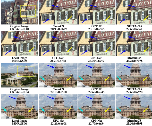
Figure 1. Visual comparisons of reconstructed image by MambaCS and other methods under Gaussian noise \delta = 0.008 at CS rates \tau \in \{0.10, 0.04\} .
