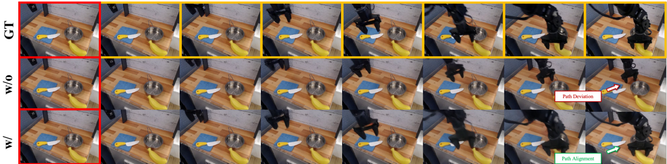
Figure 14. Ablation Results of Depth Condition Map . Without any physical controls, the robot gripper fails to act accurately aligned with the 3D action instructions, due to the accumulation of errors. While ours performs correctly, along with the entire sequence.
