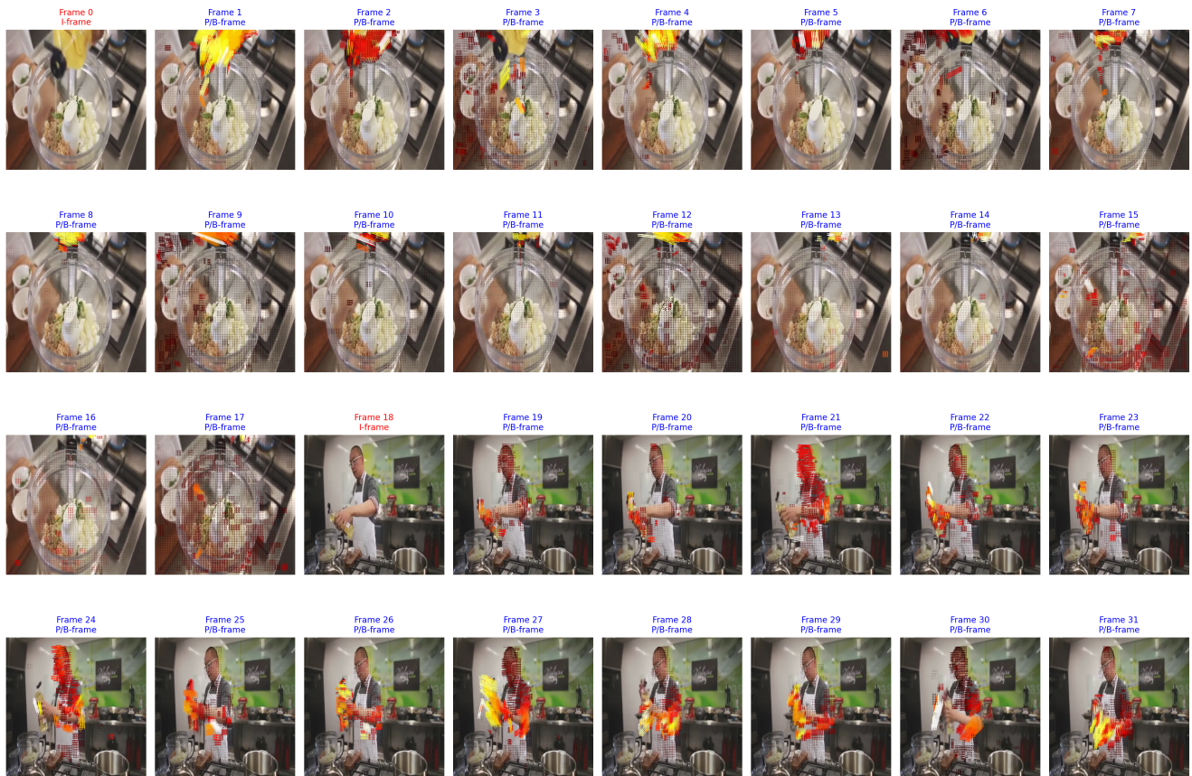
Figure 5. Example of scene-aware video preprocessing. Frames 0 and 18 are scene-adaptive I-frames used as keyframes, and the remaining frames are P/B-frames with overlaid codec motion vectors.
