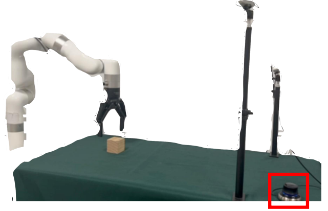
Figure 1. Real-world workspace setup for human-in-the-loop data collection. The human operator provides online correction through a 3Dconnexion SpaceMouse (marked with a red box) while monitoring the robot's execution.
