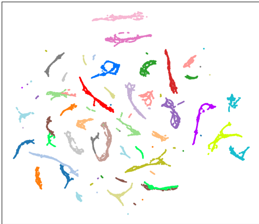
Figure 5. UMAP visualization of the global latent representations g(T_k) obtained when not enforcing the IFA loss, each color represents the global latent representations of one task.
