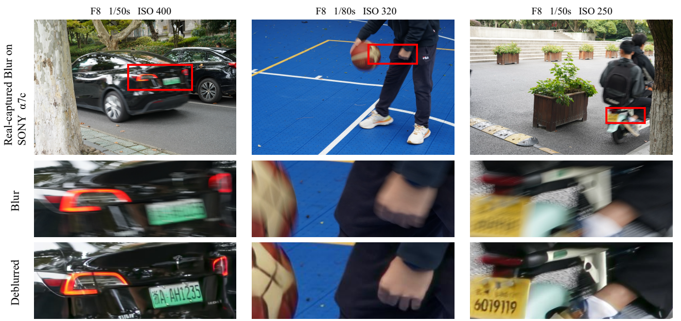
Figure 11. Deblurring results of OMDNet on real-captured blurry images. The images are taken using a SONY \alpha 7c camera with a 50 mm prime lens. Capture parameters are listed above each image.
