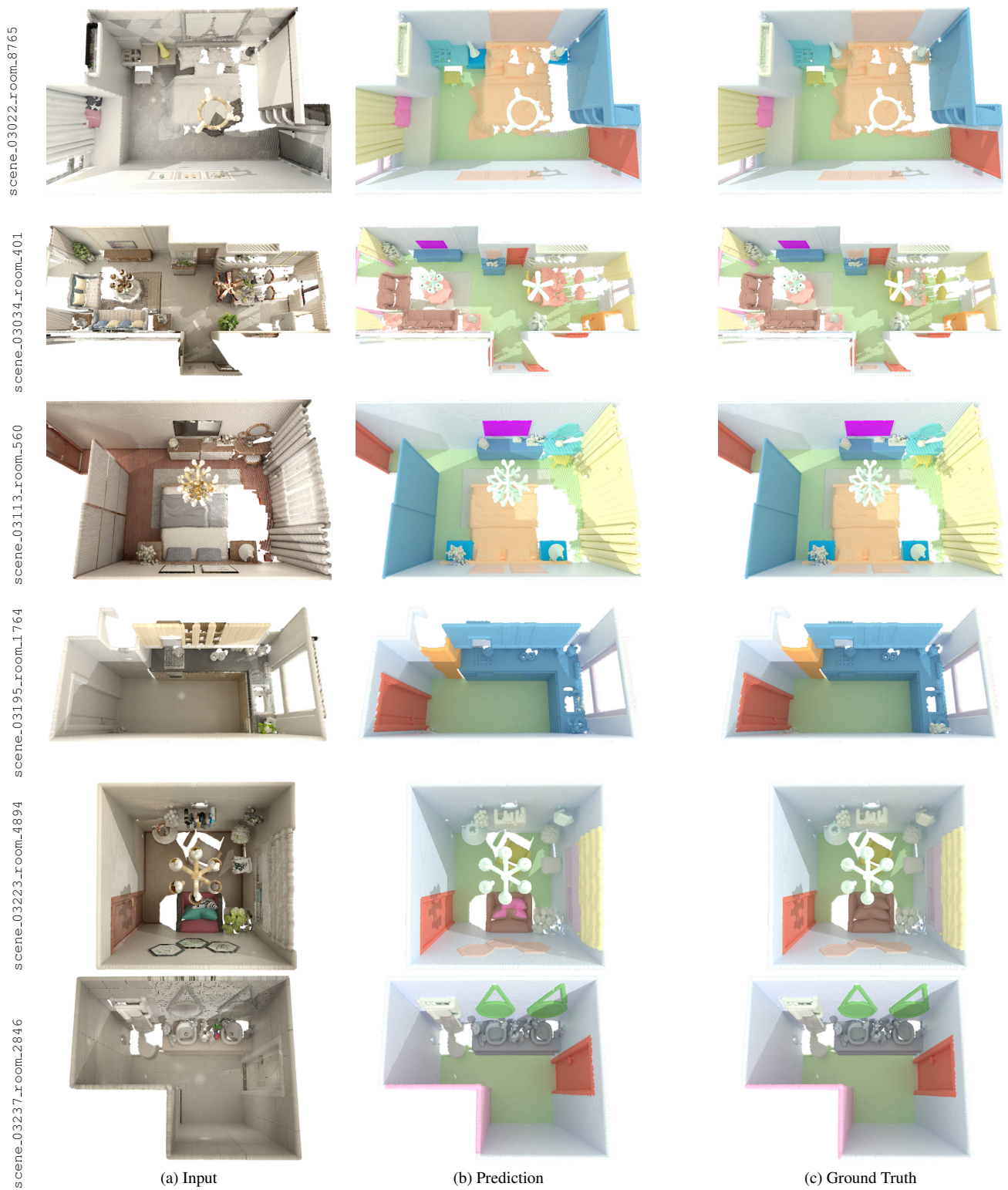
Figure 7. Structured3D semantic segmentation. We present various scenes of the Structured3D validation set: the input point cloud, the semantic segmentation from LitePT-S, and the corresponding ground truth.
