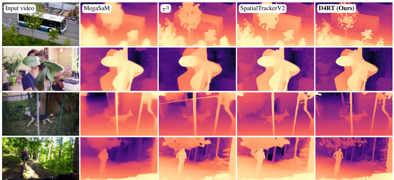
Figure 13. Qualitative depth comparison across methods – D4RT is able to perform dense depth estimation with finer details than current state-of-the-art methods, preserving geometric accuracy even in scenarios with large motion blur.
