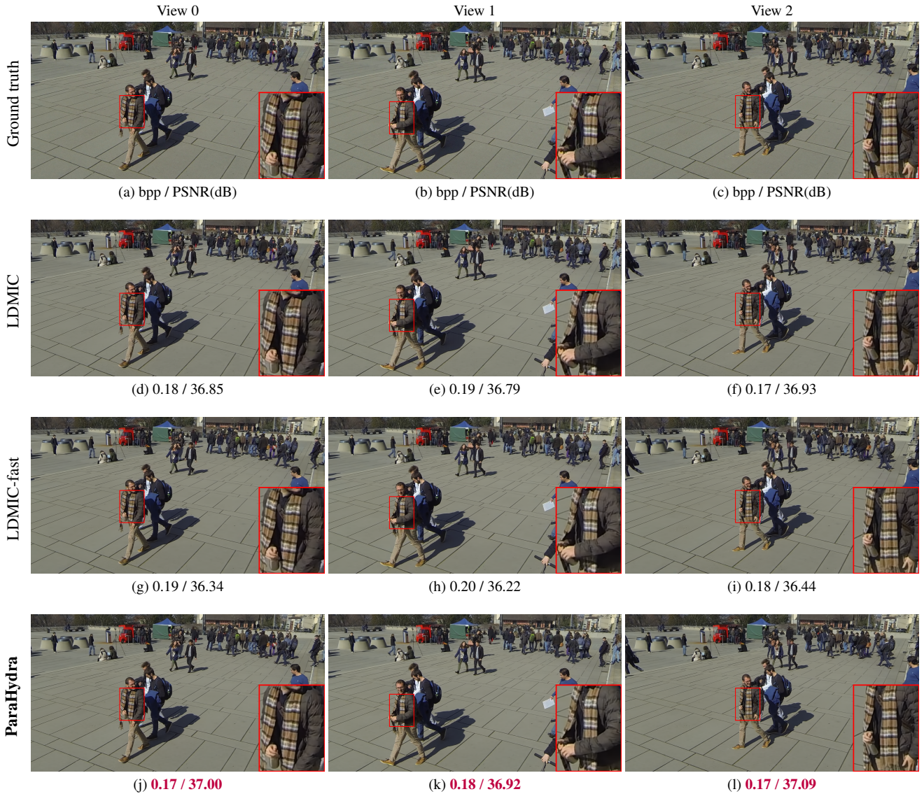
Figure 6. Qualitative comparison on the WildTrack dataset. Reconstructions from three camera views are shown with their corresponding bpp and PSNR values. Red boxes denote zoomed-in regions for detailed visual inspection. The best result is highlighted in bold .
