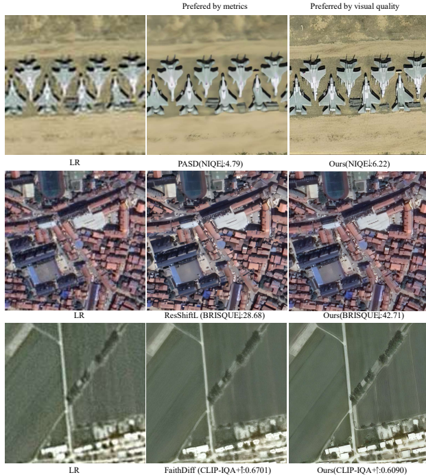
Figure 7. Here are some examples that illustrate the mismatch between no-reference metrics and visual quality. Our method produces higher-quality details, yet obtains worse no-reference scores.
