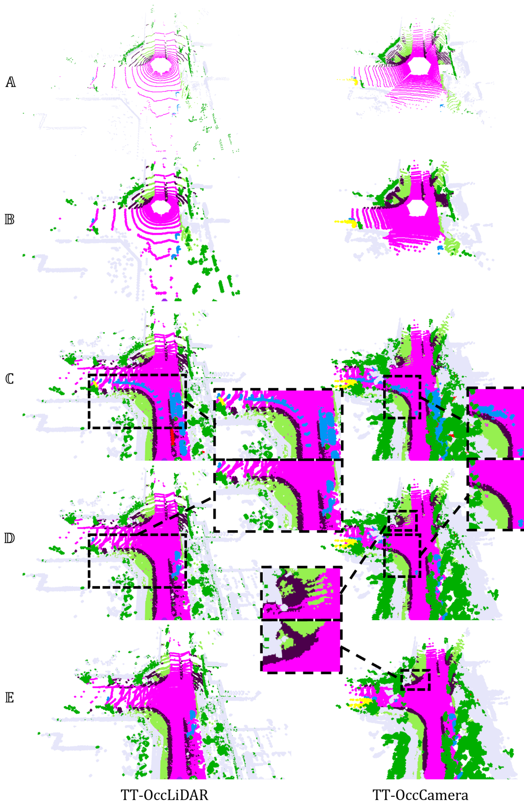
Figure 6. Zoomed-in visualization of different baselines of both variants of TT-Occ. A: Baseline. B: Covariance-aware Voxelization. C: Inherit Previous Gaussians. D: Track Dynamic Gaussians. E: TRBF Fusion.
