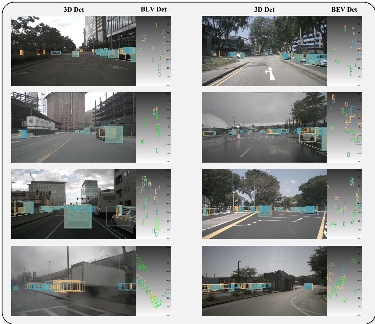
Figure A4. nuScenes frontal Visualization. MonoCoP demonstrates superior performance in both 3D and BEV detection over the baseline [80]. By predicting 3D attributes conditionally to mitigate instability and inaccuracy arising from their inter-correlations, MonoCoP predicts more accurate 3D angle and depth, demonstrating effectiveness of MonoCoP. [Key: MonoCoP, Baseline, Ground Truth]
