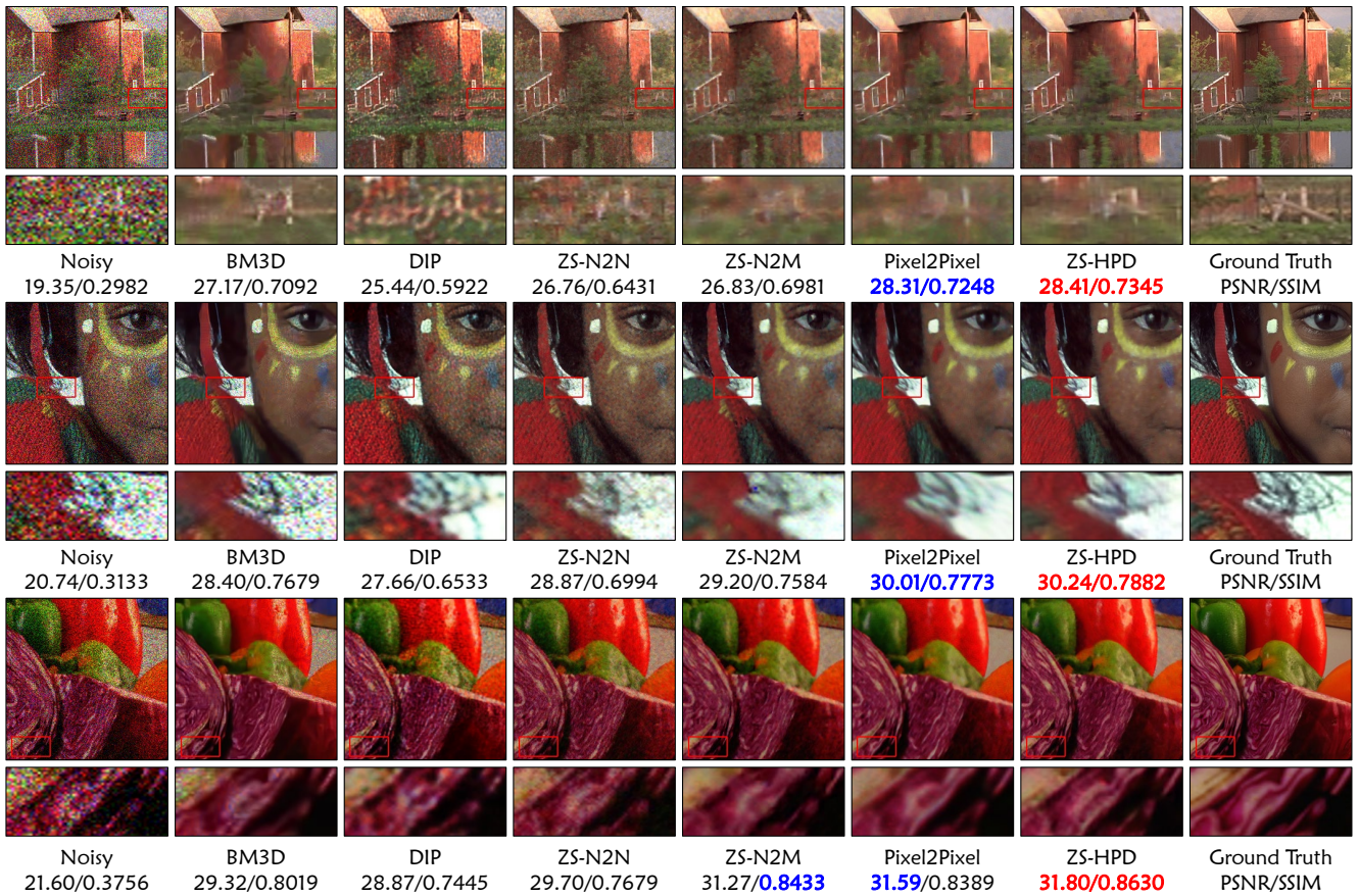
Figure 5. Visual results of several compared methods on three testing images from Kodak24 and McMaster18 with Poisson ( \lambda = 10 ) noise. The best and second-best PSNR and SSIM results are highlighted in red and blue, respectively.
