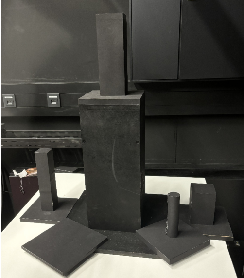
Figure 10. A set of wooden stand supports utilized for object capture. All stand supports are covered by black matte paper to eliminate color bleeding and specular reflection effects during capture.
