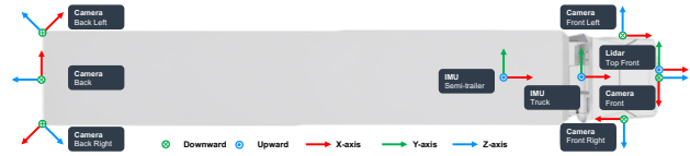
Figure 2. Placement of the sensors and their corresponding coordinate systems from a top-down view perspective
