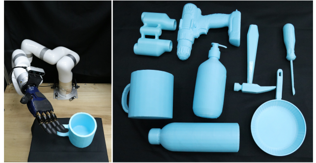
Figure 10. Real-world robotic platform. (Left) A real robotic platform comprises an XArm7 robot and a Freedom five-fingered dexterous hand. (Right) 8 real objects are used for evaluation.
