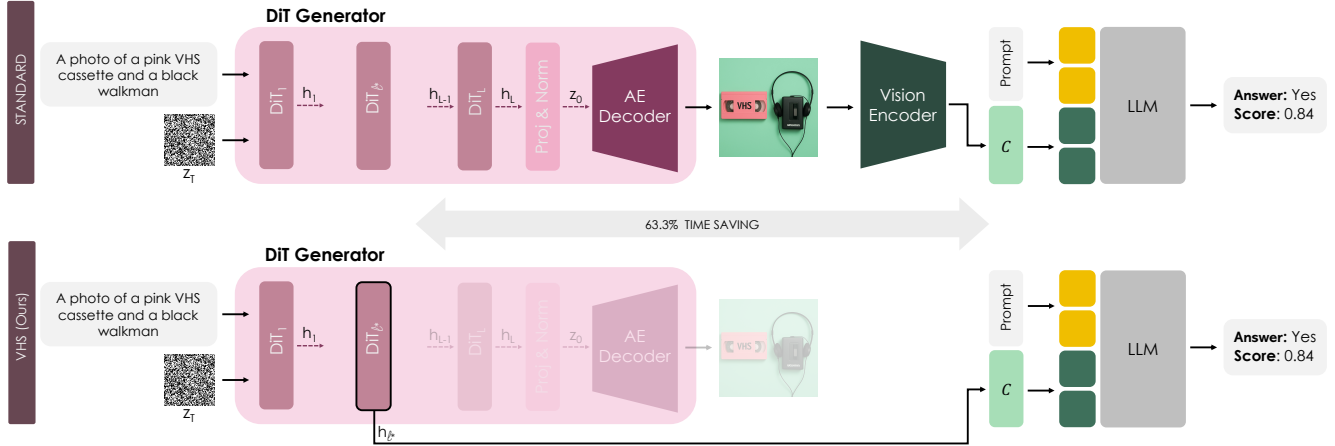
Figure 2. Comparison between a standard generation-verification pipeline (top) and VHS (bottom). VHS consumes visual features directly from the hidden states of the generator, bypassing subsequent DiT layers, autoencoder (AE) decoding, and CLIP-based re-encoding, significantly reducing sampling and verification overhead.
