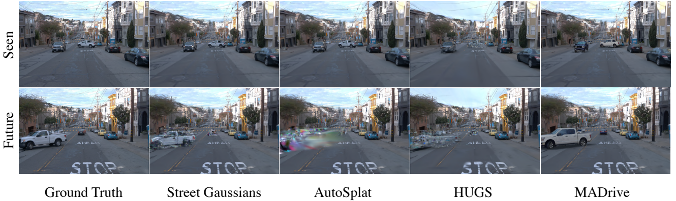
Figure 4. Qualitative comparison of MADRIVE with non-retrieval-based driving scene reconstruction methods. Reconstruction of the training views (Top). Reconstruction of the hold-out (future) views (Bottom).
