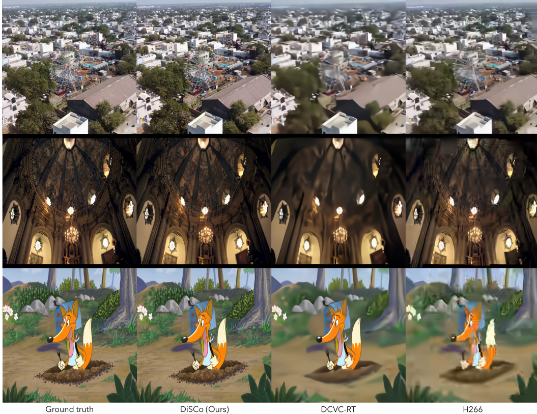
Figure 5. Visualization of compression results at 0.005 BPP (Bits Per Pixel). Zoom in for details.
