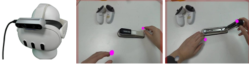
Figure 2. VR hardware and interfaces. The headset tracks the fingers and renders the tracking points as red points.
