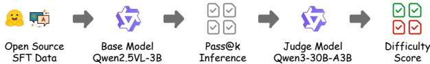
Figure 3. Illustration of pass@k data filter. The difficulty score is aligned with the number of correct answers for pass@k inference.
