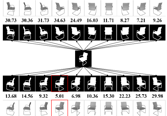
Figure 3. Visualization of Chamfer Distances. This illustration shows the chamfer distances between the query mask and 20 reference masks with their corresponding reference images. The bold numbers indicate the computed distances, and the reference pair with the smallest distance is highlighted with a red bounding box.
