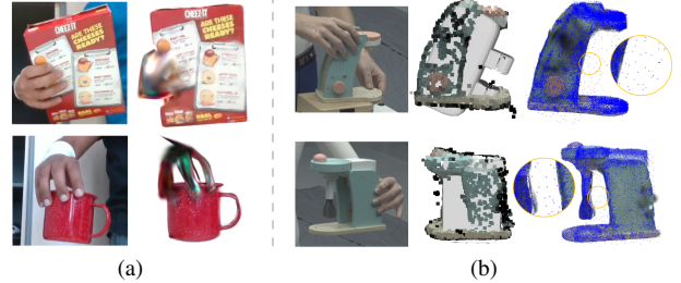
Figure 12. a) Applying \mathcal{L}_{bkg,h} for object reconstruction fails when the hand never changes its contact point with the object. In that case, unwanted gaussians spawn in the hand region. b) In some cases, the retrieved geometric prior \mathcal{O} does not align perfectly with the initial object's point cloud \mathcal{P}_{sfm} (Middle column). The results of applying \mathcal{L}_{geo} in this case will result in moving gaussian centers c_o towards unwanted regions (see blue point cloud).
