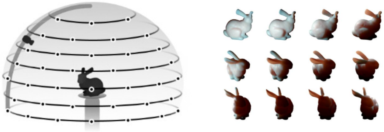
Figure 9. Overview of OLAT capture setup. A hemispherical lighting rig sequentially illuminates the object with one light at a time, capturing per-light images from fixed viewpoints.
