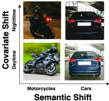
Figure 3. This figure illustrates the distinction between semantic and covariate shifts. Motorcycles and Cars represent distinct semantic categories; their inherent meaning (category) remains unchanged even when external input conditions, such as lighting, undergo a covariate shift.
