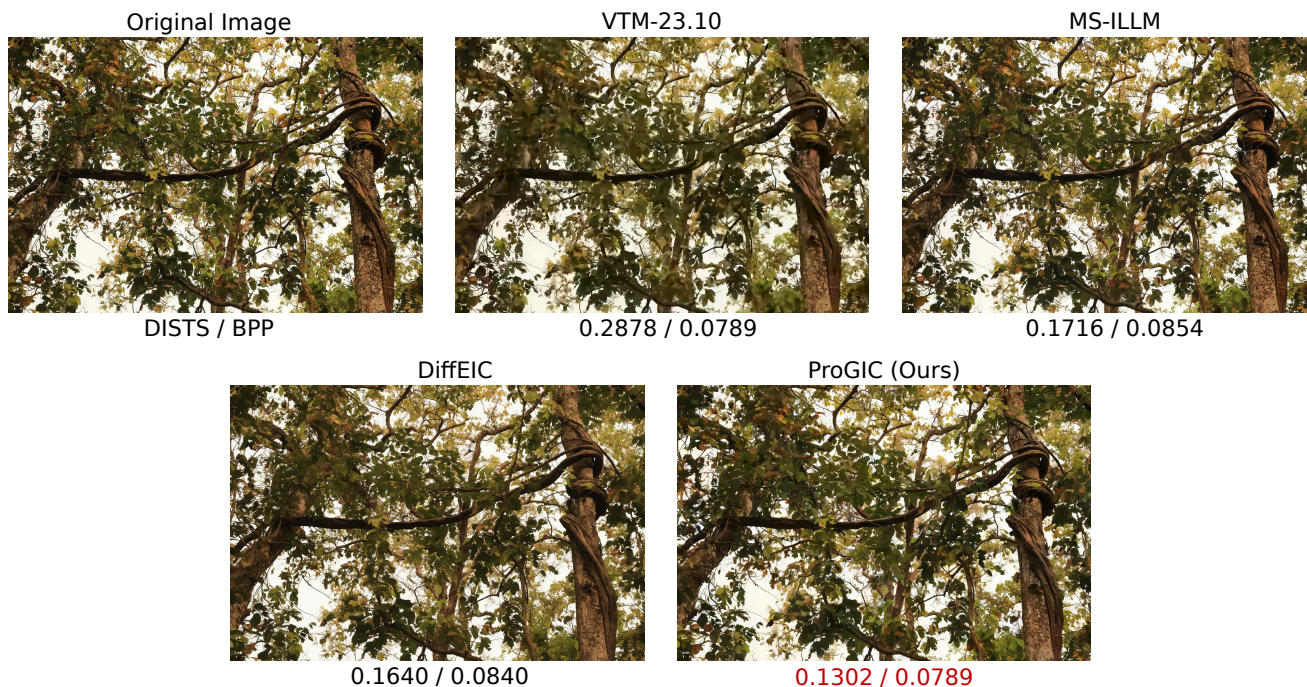
Figure 11. Visualization of reconstructed images from different methods on DIV2K. Values denote DISTS / BPP. Lower DISTS indicates better perceptual quality, and lower BPP indicates higher compression.
