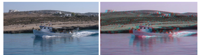
Figure 4. Stereo view synthesis. Our 3D representation enables novel view synthesis for stereo visualization from monocular video. This demonstrates that Adaptive Gabor primitives in orthographic camera coordinate space capture accurate 3D geometry, enabling immersive applications.
