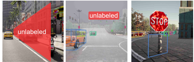
Figure 6. Label Flaws. Bench2Drive exhibits incomplete and erroneous 3D bounding box annotations in various scenes.
