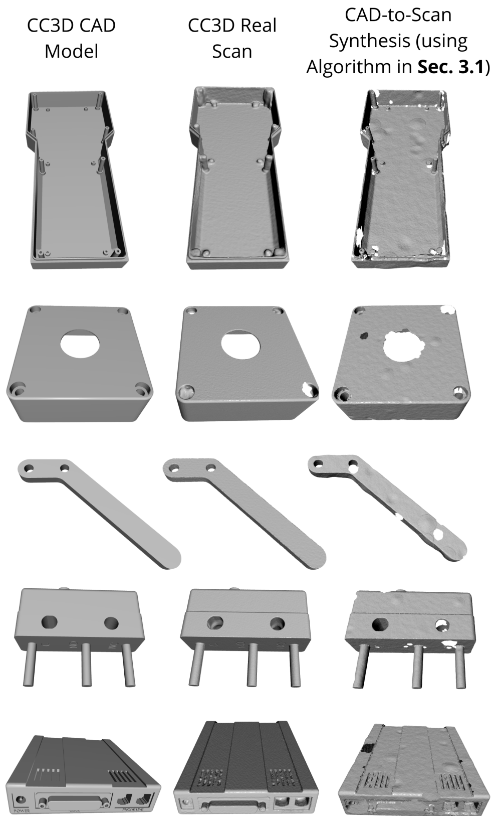
Figure 5. Visual comparison between CC3D [2] CAD models, its real scan pairs, and synthesized scans from CAD (ours)
