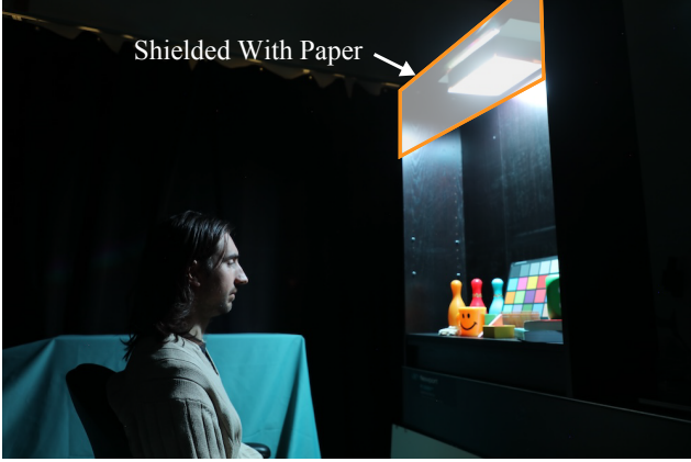
Figure 6. Our experimental setup shows a participant observing the optimized lighting patterns. Shielding prevents direct light exposure, allowing participants to observe the flicker indirectly through reflected light only.
