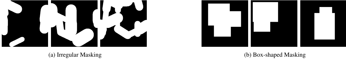
Figure 5. Masking Strategy (a) Irregular masking is implemented using random brush strokes and (b) box-shaped masking produces rectangular masked regions.
