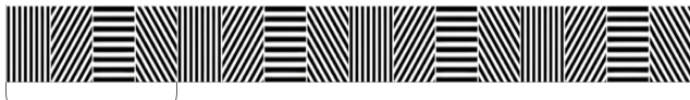
Figure 1. Illustration of our polarization mask, containing four repetitions of striped polarizers at orientations 0^\circ , 45^\circ , 90^\circ , and 135^\circ
