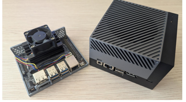
Figure 1. Edge AI Devices: NVIDIA Jetson Nano (left) - NVIDIA Jetson AGX Orin (right)
