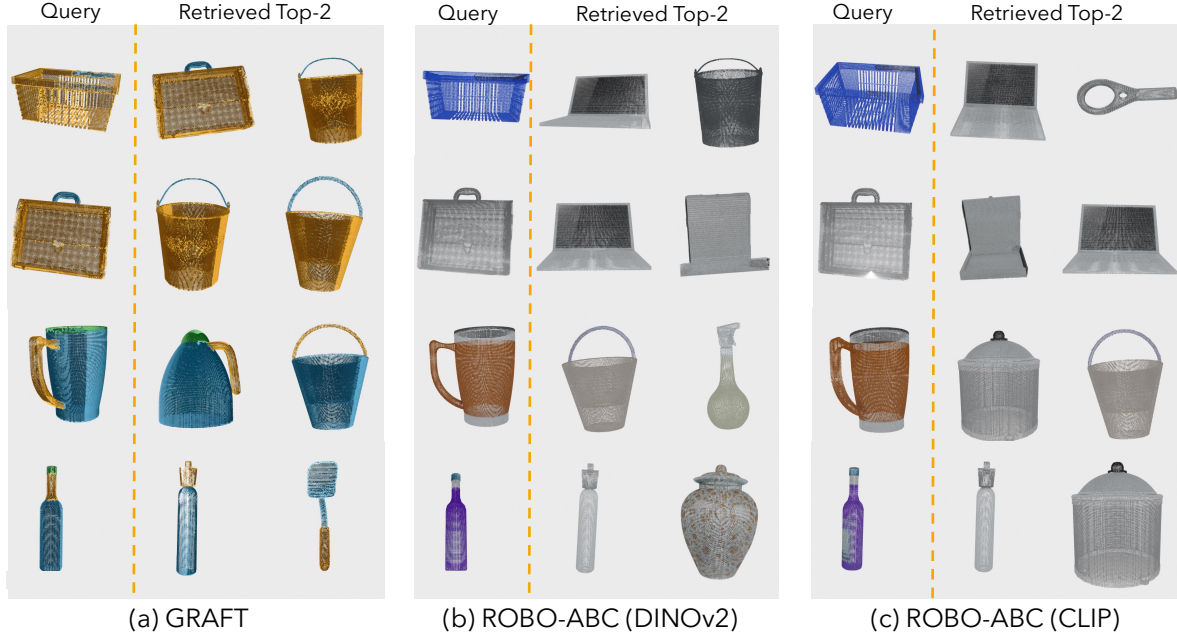
Figure 2. Top-2 retrieval results visualization for lifting task. For each query object (left), we show the two most compatible source objects retrieved by each method. GRAFT consistently retrieves functionality compatible objects whose graspable regions align with the intended manipulation.
