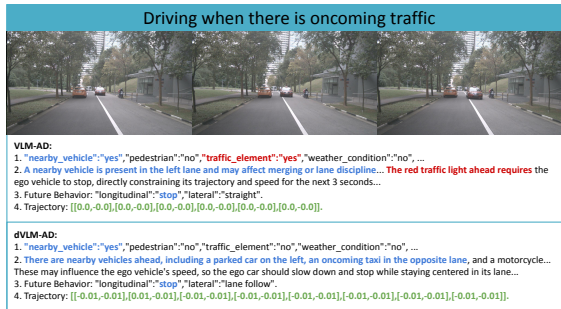
Figure 6. Scenario with oncoming traffic, where dVLM-AD’s reasoning process is more accurate with less hallucination.
