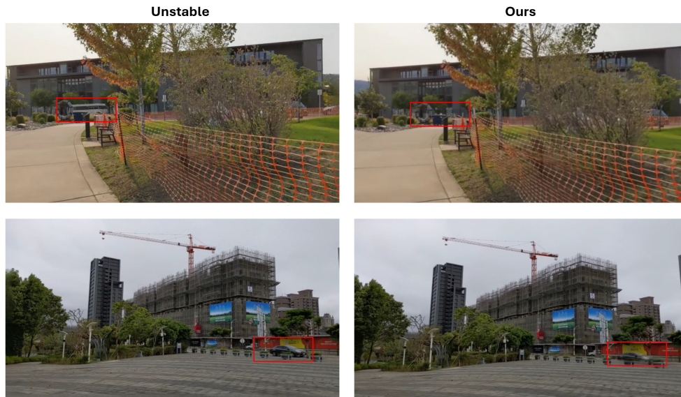
Figure 6. Dynamic Object Case: dynamic elements such as vehicles (red boxes) are either poorly reconstructed or eliminated due to the static-scene assumption.
