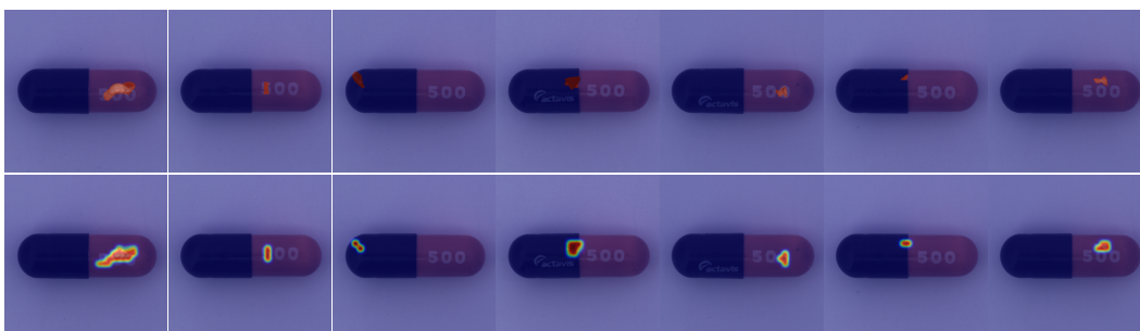
Figure S2. Segmentation results on the capsule class from MVTec-AD. Ground truth regions are marked in red (top row), and predicted anomaly maps are shown below.
