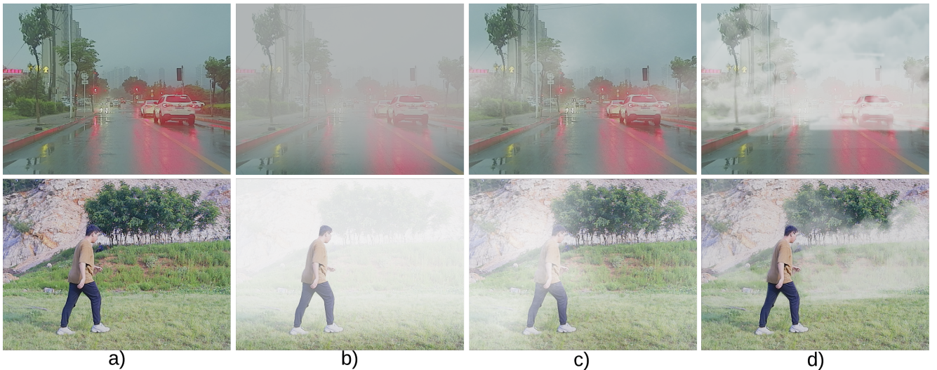
Figure 2. Visual comparison of synthetic haze generators. (a) Clean images from M3FD, (b) augmented with Synt. Haze [6], (c) augmented with HazeFlow [4], and (d) augmented with our proposed non-homogeneous pipeline. Our method generates diverse, cloud-like textures and spatially varying densities, which is crucial for emulating the irregularity of real-world atmospheric conditions.
