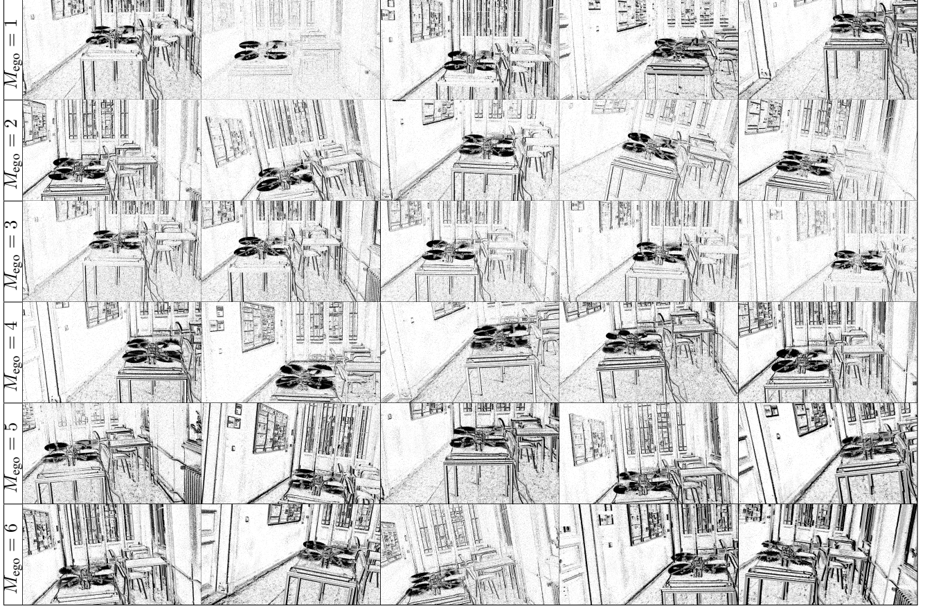
Figure S3. Aggregated events from all sequences in the Timestamped Quadcopter with Egomotion dataset with camera-to-quadcopter distance of 4 m, from the smallest (top row, M_{\text{ego}}=1 ), to the largest (bottom row, M_{\text{ego}}=7 ) egomotion intensity. Events from the first 10 ms of five 1-second intervals are shown. Positive events displayed in black, negative in gray.
