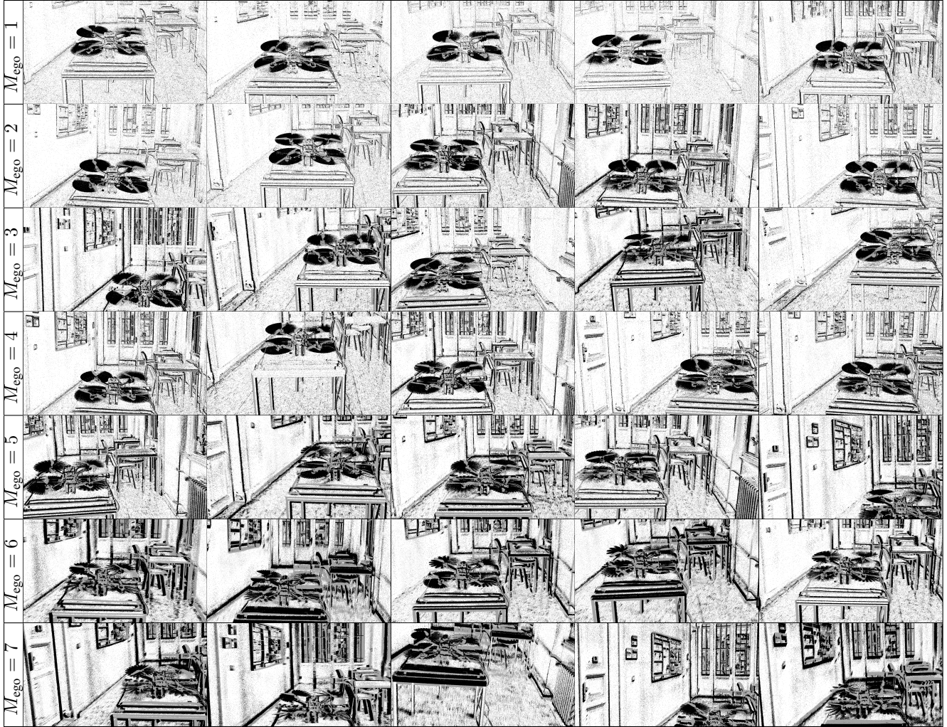
Figure S2. Aggregated events from all sequences in the Timestamped Quadcopter with Egomotion dataset with camera-to-quadcopter distance of 2 m, from the smallest (top row, M_{\text{ego}}=1 ), to the largest (bottom row, M_{\text{ego}}=7 ) egomotion intensity. Events from the first 10 ms of five 1-second intervals are shown. Positive events displayed in black, negative in gray.
