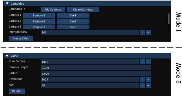
Figure 34. Generate the Video. The user is enabled to generate videos either by orbiting the camera’s center of rotation or by following a user-defined camera trajectory.
