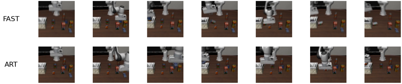
Figure 7. Qualitative comparison under jittering . The instruction is “Pick up the nearest item in the basket.”. Strong motion jittering introduces temporal inconsistencies that confuse FAST and lead to unstable grasps. By invoking the jitter correction model, ART obtains a more consistent observation stream and reliably selects the nearest item in the basket.
